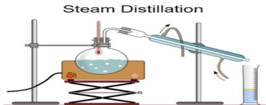
Figure 2: Steam distillation apparatus
